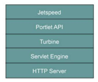
This figure illustrates the Jetspeed architecture model. Jetspeed is built on top of Turbine, a servlet-based framework, which is also part of the Jakarta Apache Project. Turbine handles user authentication and page layout as well as scheduling. Jetspeed can run on a number of servlet engines and databases. This tutorial uses Tomcat 3.2 for the servlet engine and Web server.
